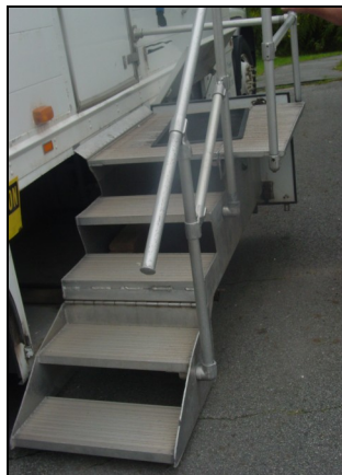
Slide out stair system offers increased safety and useable space inside coach
